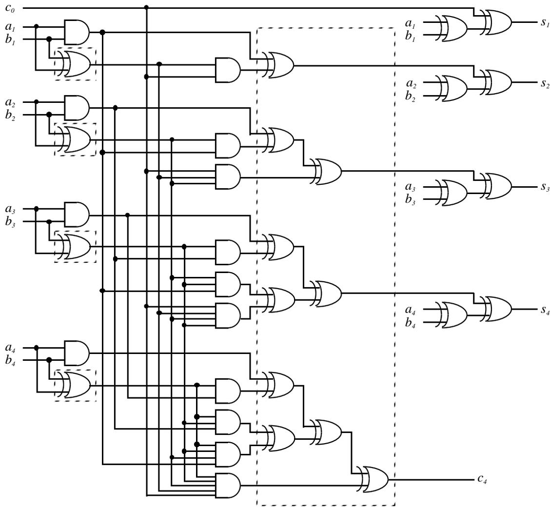
Fig. 3B: 4 bit carry look-ahead adder using AND, EXOR gates
