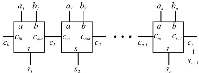
Fig. 2: Ripple carry adder
