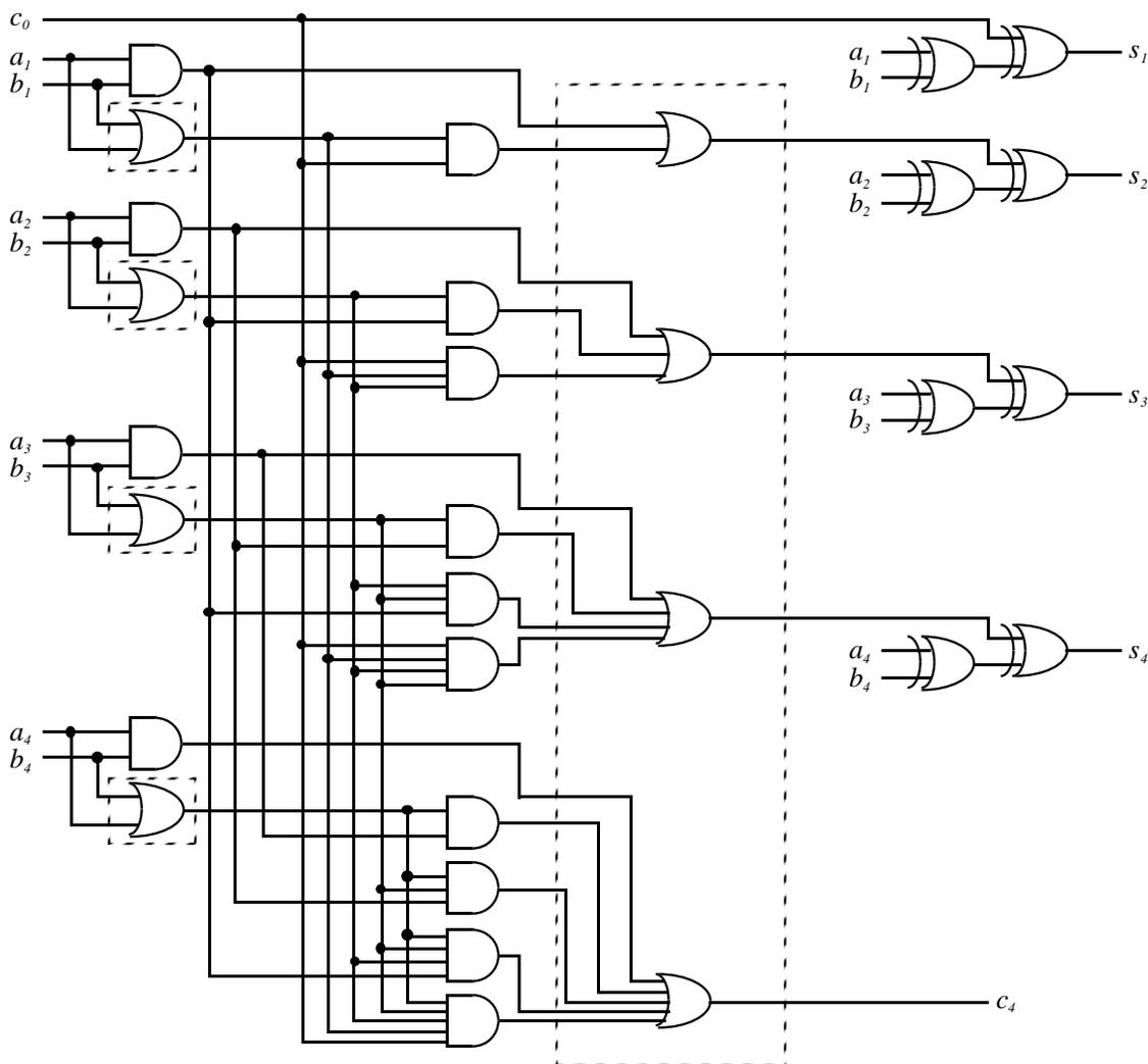
Fig. 3A: 4-bit carry look-ahead adder using AND, OR, EXOR gates
