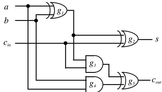
Fig. 1B: Full adder using AND, EXOR gates
