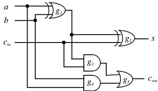
Fig. 1A: Full adder using AND, OR, EXOR gates
