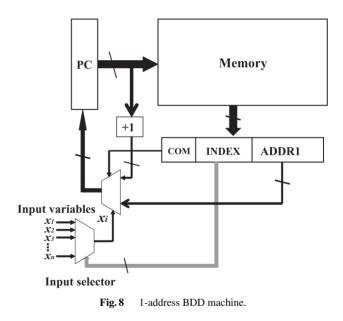
is specified. To reduce the width of the instruction words, 1-address BDD machines shown in Fig. 8 have been developed [6], [11], [18], [33]. In this case, when the value IN-DEX is 1, the machine works similarly to the case of the 2-address BDD machine. Otherwise, the content of the program counter (PC) is incremented by one, to access the next address. In this case, the size of the instruction word is reduced, but unconditional GOTO instructions are necessary, as shown later.
