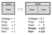
Fig. 1 Using a dual core processor to reduce the power by half.
