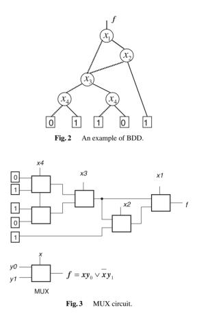
Parallelization can be implemented by multi-way branching programs. Thus, performance can be improved without increasing the clock frequency.
